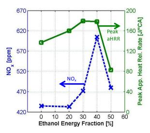
Figure. 6.  $NO_x$  emission and peak apparent heat release rate for various ethanol energy fractions (diesel injection at -3° CA aTDC)
