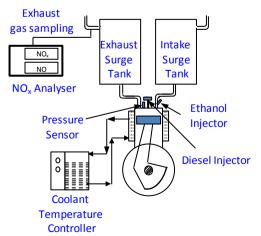
Figure 1. Schematic diagram of experimental facility
