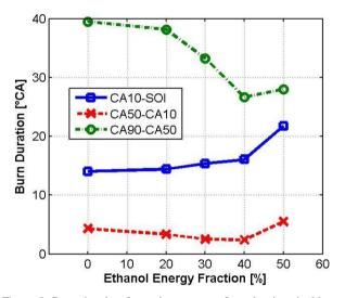
Figure 5. Burn duration for various stages of combustion: ignition delay (CA10-SOI), initial burning (CA50-CA10), late cycle burning (CA90-CA50) at different ethanol energy fractions (diesel injection at  $-3^{\circ}$  CA aTDC)
