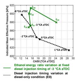
Figure 4. Indicated mean effective pressure (IMEP) against CA50 for dual-fuelling and diesel only operation
