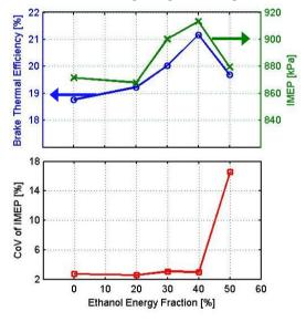
Figure 3. Indicated mean effective pressure (IMEP) and coefficient of variation of IMEP for different ethanol energy fractions (diesel injection at -3° CA aTDC)
