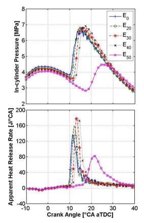
Figure 2. In-cylinder pressure (top) and apparent heat release rate (bottom) for different ethanol energy fractions (diesel injection at  $-3^{\circ}$  CA aTDC)
